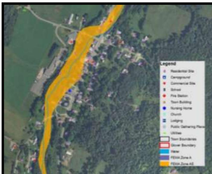
Figure 12: Zone AE and structures within Glover Village
